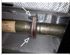
On Malibu models only: Separate exhaust flange and carefully slide the exhaust forward out of the rear bumper exhaust hangers. Set aside exhaust for later reinstallation. Remove the inside lower bumper bolts on each side of the vehicle using a 15mm socket. Replace with the supplied M10 bolts.
