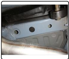
2. Enlarge access holes and fishwire 1/2" carriage bolts and CM-SP6 spacers into position and reverse fishwire remaining 1/2" carriage bolts and CM-SP6 spacers into access hole. Leave fishwires attached.
