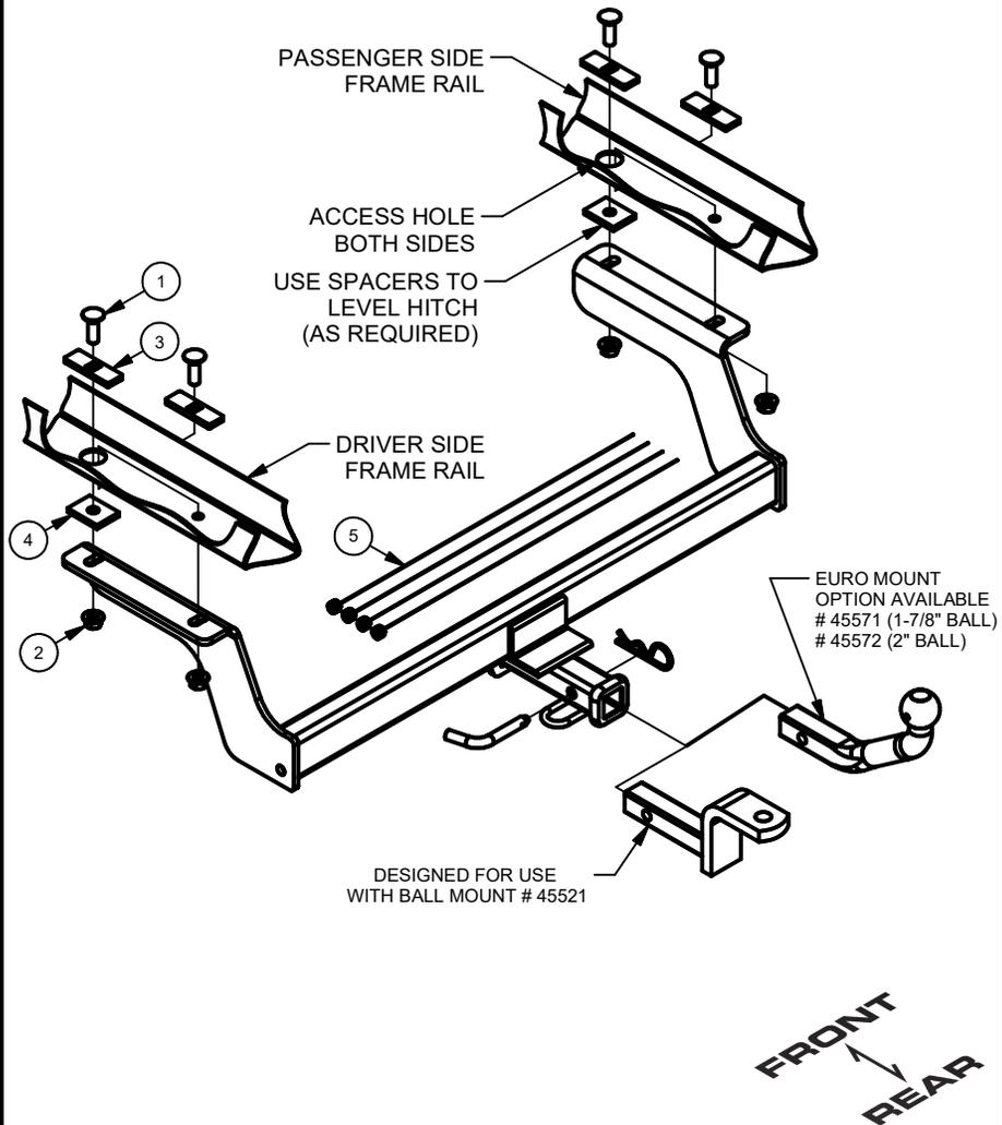
1. Remove (2) rubber plugs from each frame rail and return to vehicle owner (leave center plugs in the frame).
