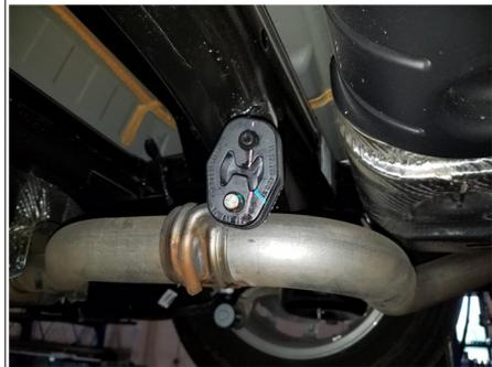
4. Locate and remove (2) plastic nuts with a 10mm socket. Remove heat shield and mark out a 5" x 13" section with masking tape. Use aviation shears to trim marked area. Reinstall with (1) nut using a 10mm socket.
