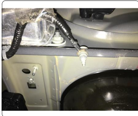
9. Raise hitch into position starting with the passenger side. Run the fishwires through the holes on hitch to help align bolts with hitch holes. Remove fishwires and loosely fasten (2) 1/2" hex nuts on driver side and (3) 1/2" hex nuts on passenger side.
