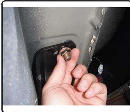
5. Torque all 12mm hardware to 86 lb-ft and all 7/16" hardware to 59 lb-ft. Reinstall exhaust deflector.
