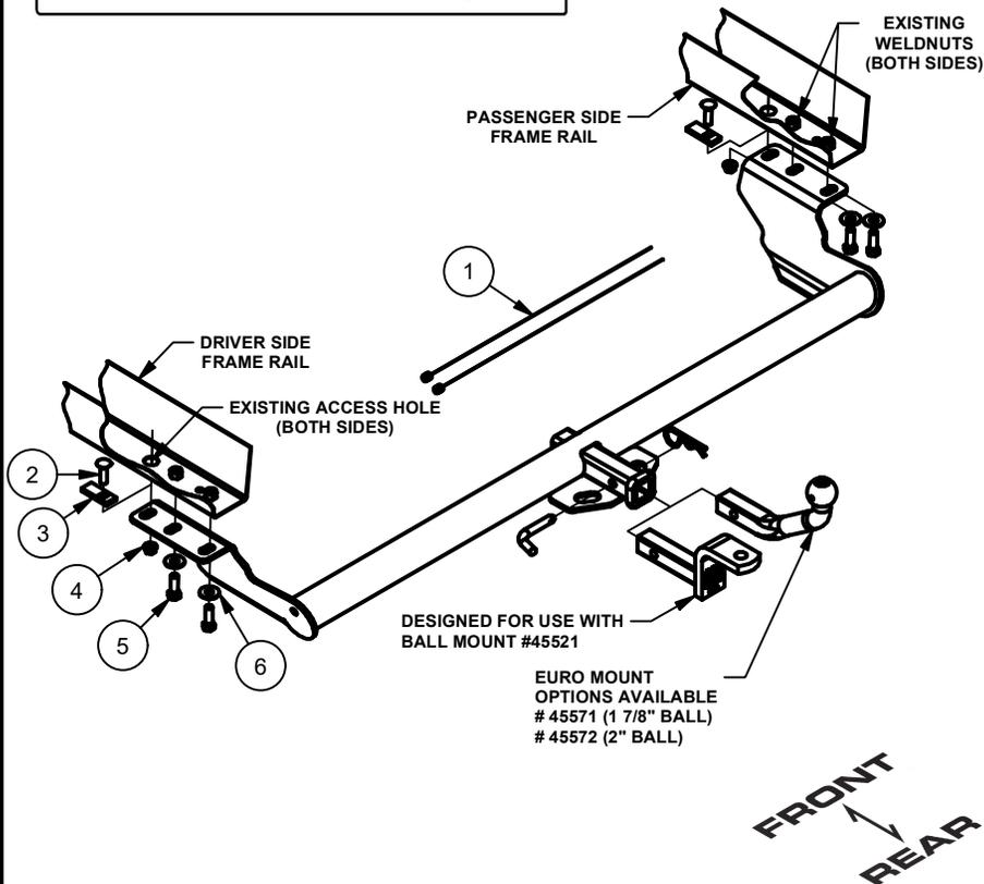
1. If present, remove (6) fasteners ((4) plastic push pins, (1) phillips head screw and (1) hex bolt with 10mm socket) and the plastic underbody panel covering the driver side frame rail. Return fasteners and plastic shield to owner. Remove (2) fasteners on the exhaust deflector and temporarily remove deflector.
