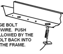
ATTACH FISHWIRE TO CARRIAGE BOLT AND SLIDE SPACER ONTO FISHWIRE. PUSH THE BOLT THRU THE HOLE FOLLOWED BY THE SPACER (AS SHOWN). PULL BOLT BACK INTO POSITION, PROTRUDING FROM THE FRAME.
