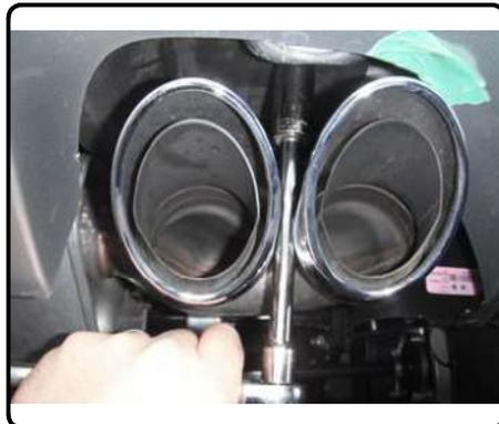
9. Reinstall or raise exhaust back into position and reinstall the flange nuts removed in step 2. Reinstall the rear bumper cover screws removed in step 1.
