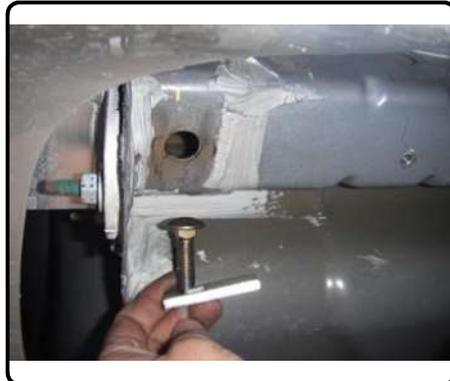
5. Using tape, a marker, and measuring tape, locate the center of the vehicle and mark a 2 1/2" side to side and 2 5/8" lengthwise cutout. Using a tin snips or aviation shears, trim out the area marked. NOTE: These dimensions are reference only, make sure to check hitch location on vehicle prior to trimming.
