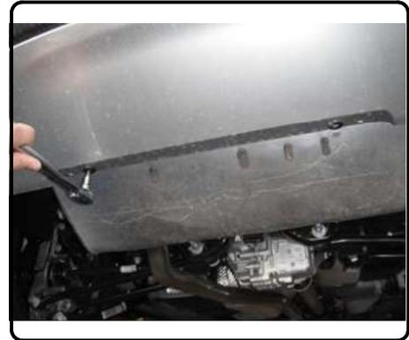
2. Use a 13mm socket to remove the (1) nut on each of the (2) rearward most exhaust hanger brackets. **NOTE:** Support the exhaust before removing the nuts to prevent damage to the exhaust.
