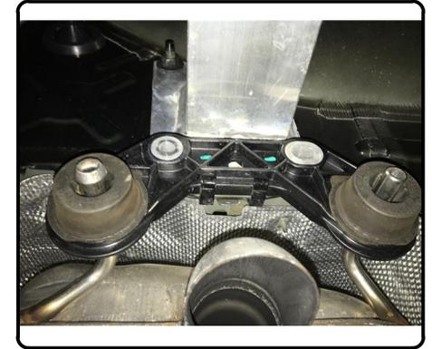
2. Remove heat shield using needle nose pliers to loosen (4) speed nuts on driver side and (2) speed nuts on passenger. Trim heat shield using aviation shears as shown in Heat Shield Trim Diagram. Reinstall trimmed heat shield.
