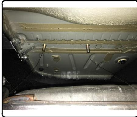
4. Remove (1) screw on each side using 7mm socket attaching rear fascia to vehicle.
