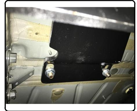
6. Reinstall vehicle exhaust bracket on hitch mounting plate and secure using (2) M10 x 70 and (1) CM-SP1 on each side.
