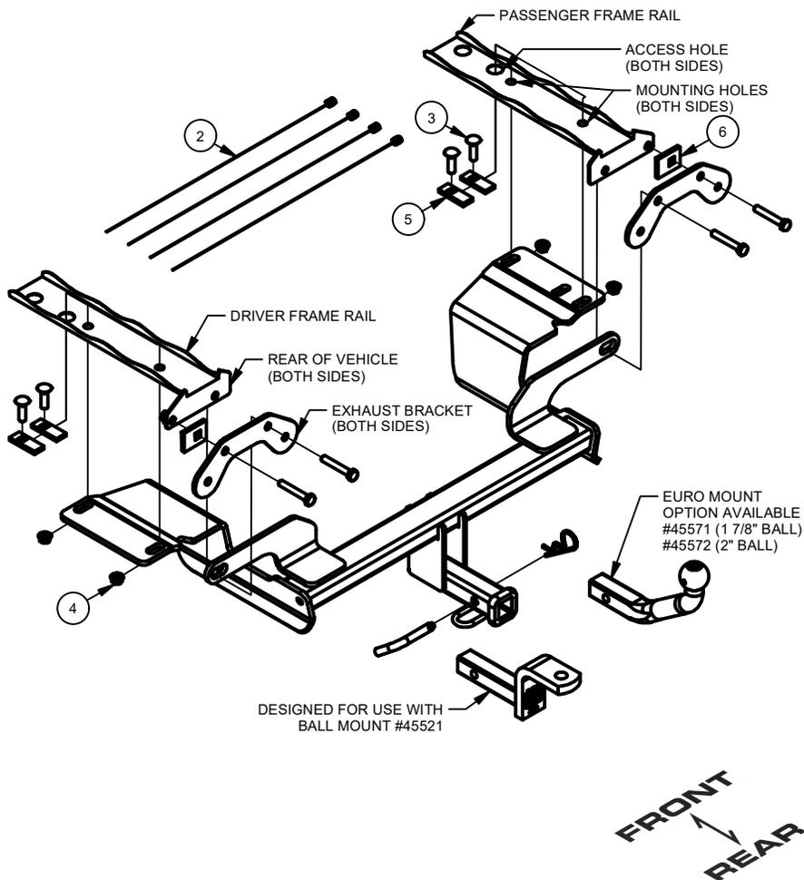
1. Lower exhaust using 15mm socket to remove (2) bolts attaching the exhaust bracket to rear of vehicle, on each side.
