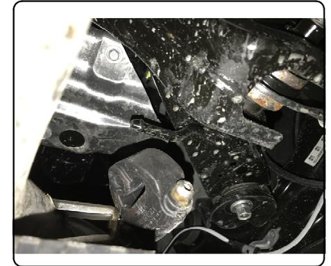
2. Fishwire (2) 7/16" carriage bolts and (2) CM-SP2 spacers through the vehicle access holes to the attachment holes on each side. See FISHWIRE DIAGRAM below.
