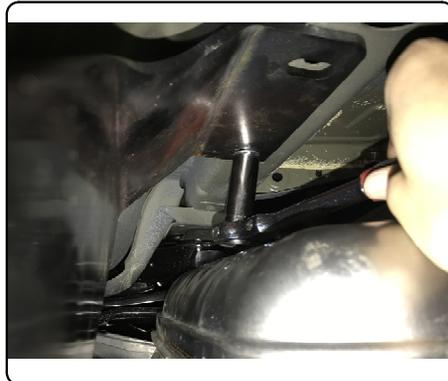
5. Torque all 7/16" hardware to 59 ft-lbs and all 1/2" hardware to 110 ft-lbs. Reinstall items removed in Step 1.
