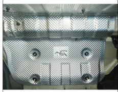
2. Clear away caulk from frame rail on both sides. Mark (1) hole 2.5" rearward of access hole centered along frame rail on each side. Raise hitch into position to use as template to mark out forwardmost holes. Lower hitch and drill (4) holes with 17/32" drill bit for 1/2" fasteners.
