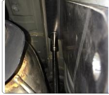
Modify heat shields as shown in trim diagram and reinstall with original fasteners. Raise exhaust and reinstall (4) rubber exhaust isolators removed in step (1).
