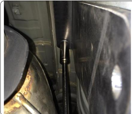
5. Modify heat shields as shown in trim diagram and reinstall with original fasteners. Raise exhaust and reinstall (4) rubber exhaust isolators removed in step (1).
