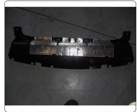
2. Lower the muffler by removing (3) exhaust hangers, (1) from each side and (1) in front of the muffler. Temporarily remove heat shield by removing (9) formed nuts with a 10mm socket.
