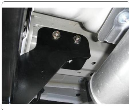
5. Torque all 7/16" fasteners to 70 lb.-ft and all 1/2" fasteners to 110 lb.-ft. Reinstall heat shield and exhaust removed in step 2.
