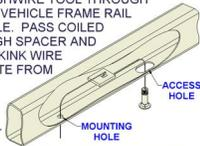
**RUBBER ISOLATOR REMOVAL DIAGRAM**
