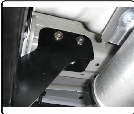
5. Torque all 7/16" fasteners to 59 lb.-ft and all 1/2" fasteners to 110 lb.-ft. Reinstall heat shield and exhaust removed in step 2.
