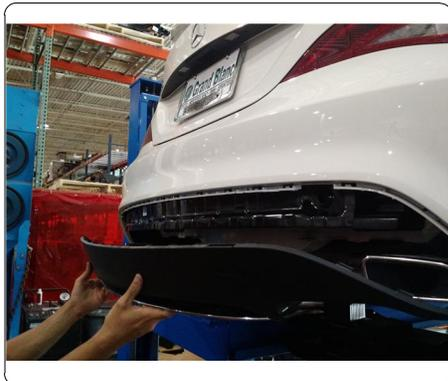
5. Locate the bumper beam connection points and remove (8) nuts, (4) from each side using a 16mm socket. Remove bumper beam by pulling bumper towards rear of car while twisting the bumper beam up towards the top of the vehicle. Set aside for later reinstallation. **NOTE:** Use silicone sealant around openings of the frame rail on each side as shown in FIGURE 1.
