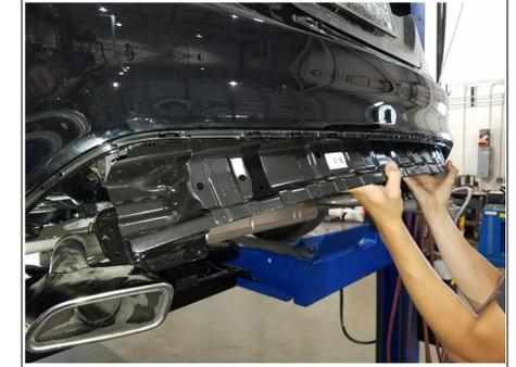
6. Place bumper beam onto hitch aligning the studs with the holes on the hitch. Raise hitch into position with the bumper beam, tucking them underneath the bumper fascia and then twisting bumper beam to reinstall. Loosely fasten using nuts removed from Step 5.
