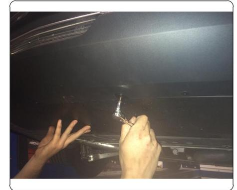
2. Pull back wheel well cover to remove (4) screws (2) on each side using 7mm socket.
