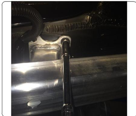
9. Trim underbody panel as shown in the trim diagram using aviation shears.
