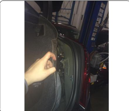
5. Gently remove rear bumper fascia by releasing the press-in tabs along top portion of bumper fascia. Unclip motion sensor harness. Set aside for reinstallation.
