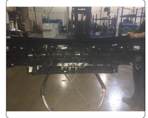
6. Remove the bumper beam by removing (2) nuts and (2) bolts using 13mm socket, on each side. Set aside bumper beam for reinstallation.
