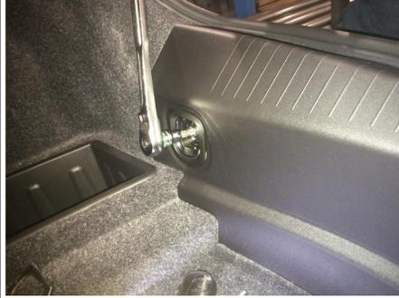
4. To access taillight removal, remove (4) plastic clips, (2) on each side. To remove taillights, pull back trunk carpet locate and remove (8) nuts using 8mm socket, (4) on each side. Unclip electrical harness and gently remove taillight, set aside for reinstallation.
