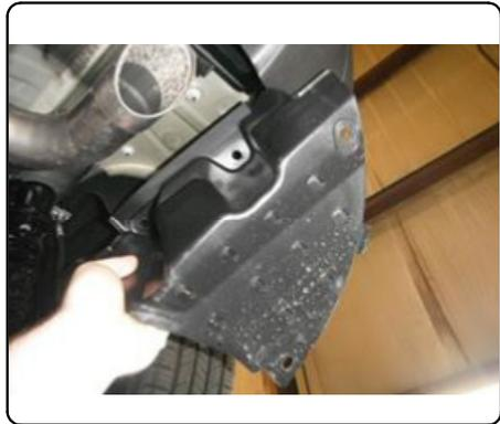
2. Lower exhaust by detaching (2) exhaust isolators.
