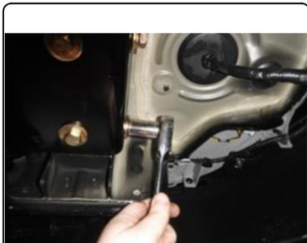
5. Raise exhaust back into position and reattach exhaust isolators removed in Step 2.
