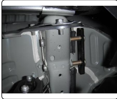
4. Raise hitch into position and slide the bolts through to support it. Loosely install the supplied hex flange nuts and the (2) hex bolts and conical washers as shown. Be sure teeth on washers are against the hitch mounting plate.
