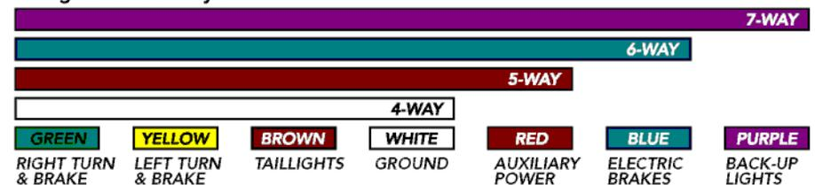
CURT DISCLAIMER: WIRING COLOR SHOWN WORK IN CONJUNCTION WITH CURT MANUFACTURING PRODUCTS.
