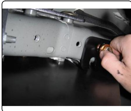
5. Torque all 10mm fasteners to 48 lb-ft and all 1/2" fasteners to 110 lb-ft.
