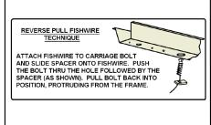
5. Raise hitch into position, threading the fishwires into the mounting holes. Remove fishwire and loosely install 1/2" Hex Flange Nuts.
