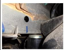
2. Enlarge the rearmost hole with the die grinder on each frame rail to allow the carriage bolts and spacers to be inserted into the frame rail.
