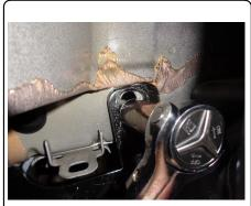
4. Fishwire (1) 1/2" carriage bolts and (1) CM-SP10 into the forwardmost holes on the outside of each frame rail. Reverse Fishwire (1) 1/2" carriage bolts and (1) CM-SP10 into the rearmost hole on the bottom of each frame rail leaving the fasteners in the fram until hitch is in position. Keep wires attached until hitch is raised into position.
