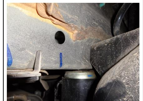
2. Enlarge the rearmost hole with the die grinder on each frame rail to allow the carriage bolts and spacers to be inserted into the frame rail.
