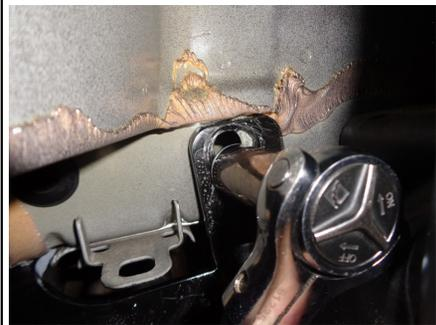
4. Fishwire (1) 1/2" carriage bolts and (1) CM-SP10 into the forwardmost holes on the outside of each frame rail. Reverse Fishwire (1) 1/2" carriage bolts and (1) CM-SP10 into the rearmost hole on the bottom of each frame rail leaving the fasteners in the fram until hitch is in position. Keep wires attached until hitch is raised into position.
