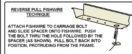
5. Raise hitch into position, threading the fishwires into the mounting holes. Remove fishwire and loosely install 1/2" Hex Flange Nuts.
