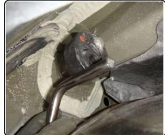
Remove the muffler heat shield and trim to clear the hitch mounting plate. (See Heat Shield Trim Diagram.)
