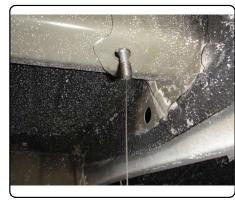
5. Raise the hitch into position. Center the hitch on the vehicle, remove fishwire, and loosely secure the hitch to the vehicle with hex flange nuts as shown.
