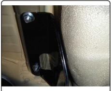
9. Reinstall the heat shield, raise the exhaust and reinstall the rubber isolators.
