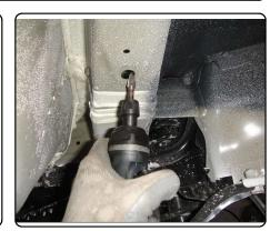
Fishwire a carriage bolt and spacer into the rearmost hole in each frame rail as shown.
