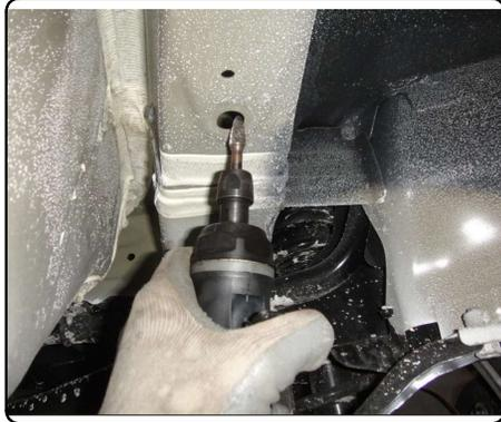
4. Fishwire a carriage bolt and spacer into the rearmost hole in each frame rail as shown.
