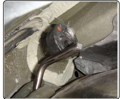
2. Remove the muffler heat shield and trim to clear the hitch mounting plate.
