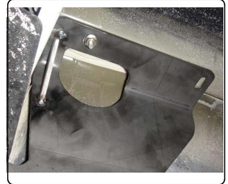
6. Using the hitch as your template mark and drill the forward holes in the frame rail. Fishwire a carriage bolt and spacer into each drilled hole and secure the hitch with a hex flange nut as shown.
