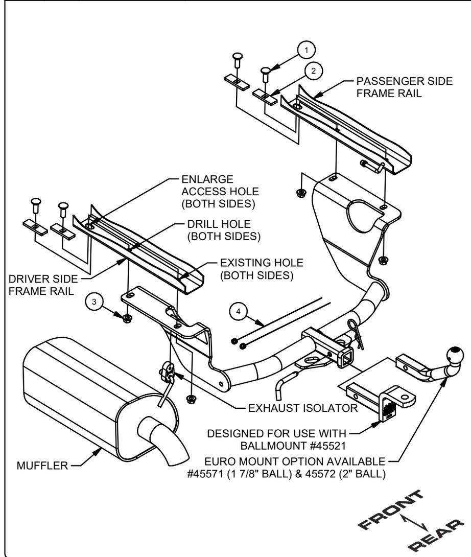
1. Lower the exhaust by removing the (3) rearmost rubber exhaust isolators from the frame mounted hangers.
