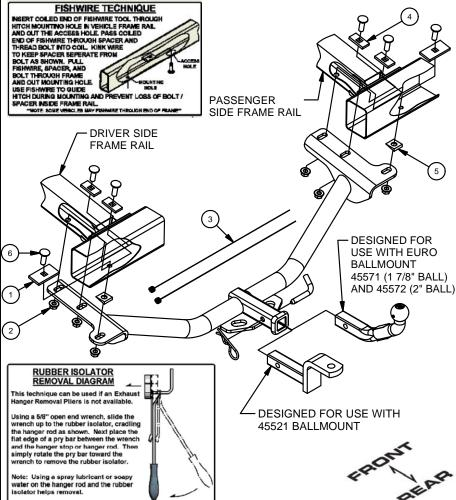
1.) Lower exhaust by removing rubber isolators (3 each side) as shown.
