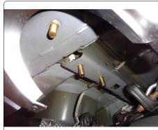
4.) Raise hitch into position with the "wedge" shaped spacers between as shown and secure with hex flange nuts.
