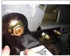
6.) Raise exhaust back into position and reinstall the (4) rubber isolators removed in Step 1.
