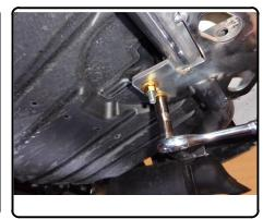
6. Torque all 1/2" fasteners to 110 lb-ft and 3/8" fasteners to 37 lb-ft.
