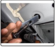
4. Drill (1) hole in each side of the frame rail for the remaining  $\frac{1}{2}$ " fastners using the hitch front mounting hole as a template. Fish remaining
