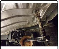
8. Move exhaust back into location, and reinstall rubber exhaust hangers.
