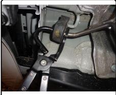
2. Remove the heat shields on each side of the car, (8) bolts using the 10mm socket.
