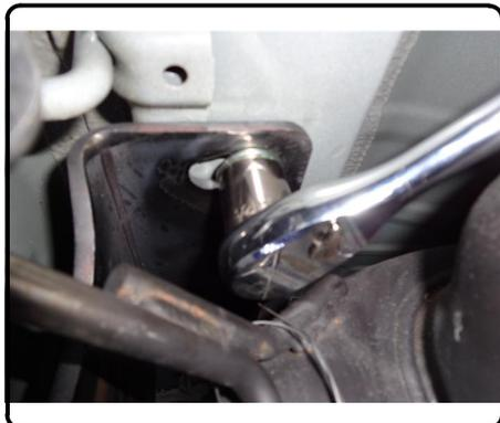
5. Install the U-bolt through the vehicle tow hook and hitch as shown below, install both washers and nuts evenly.
