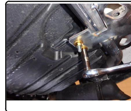
6. Torque all 1/2" fasteners to 110 lb-ft and 3/8" fasteners to 37 lb-ft.
