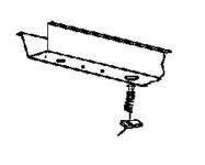
4. Raise hitch into position by loosely securing with the 1/2" hardware, and loosely secure tow loop attachment with 3/8" u-bolt, conical washers, and 3/8" nuts. Torque M8 hardware to 25 ft-lb, 3/8" hardware to 30 ft-lb, and 1/2" hardware to 110 ft-lb.
