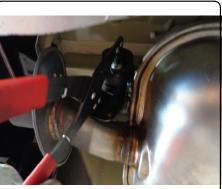
2. Unbolt exhaust hanger brackets (both sides), by removing(2) M8 nuts from each bracket. (Return bracket to customer)
