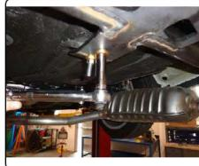
5. Raise exhaust back into position by connecting the rubber isolators on the muffler to the hanger studs on the hitch, and reconnect the center isolator. Reconnect exhaust tips removed in step (1)
