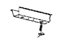
4. Raise hitch into position by loosely securing with the 1/2" hardware, and loosely secure tow loop attachment with 3/8" u-bolt, conical washers, and 3/8" nuts. Torque M8 hardware to 25 ft-lb, 3/8" hardware to 30 ft-lb, and 1/2" hardware to 110 ft-lb.
