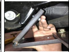
4. Assemble the bolt on bracket as shown by placing the handle nut in the suspension housing and securing with a 1/2" bolt and lock washer. (Shown below is the bolt on bracket (1) used on (FWD) vehicles built before mid year, 2013. The bolt on bracket (2) is used on all (AWD) and (FWD) models built 2013 mid year to present.)
