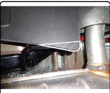
2. Raise receiver tube section of hitch into place and use the 8mm bolts and conical toothed washers provided to secure into place. Secure the 8mm nut to the back side of the frame bracket on each side to hold the exhaust bracket in place.
