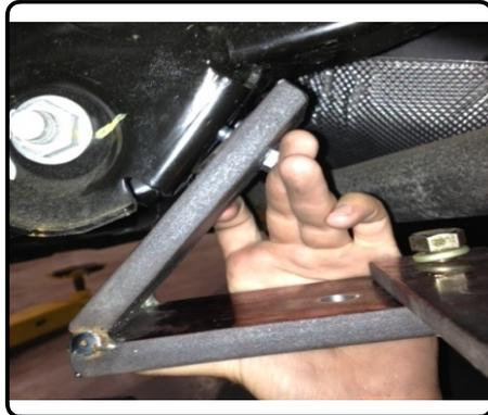
4. Assemble the bolt on bracket as shown by placing the handle nut in the suspension housing and securing with a 1/2" bolt and lock washer. (Shown below is the bolt on bracket (1) used on (FWD) vehicles built before mid year, 2013. The bolt on bracket (2) is used on all (AWD) and (FWD) models built 2013 mid year to present.)
