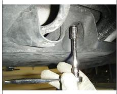
2. Begin bumper cover removal process by removing (1) screw and (1) push fastener from behind rear tire.
