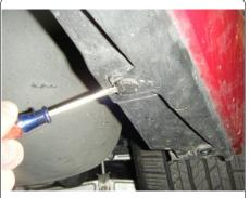
3. Remove (1) screw hidden behind the wheel well at the top of the facia. Remove the plastic clip by prying it out with a flat head screw driver.
