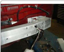
9. Raise hitch and bumper beam into position and secure to the vehicle with the M8 bolts removed in STEP 9. Torque all M8 hardware to 23 ft-lbs.
