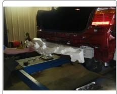
7. Remove plastic blocks from bumper beam and set aside for reinstall later.
