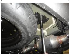
2. Lower exhaust by removing (3) rubber isolators.
