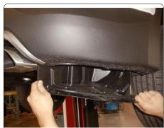
4. Raise hitch into position and secure to the existing weldnuts with M10-1.25 x 25mm bolts and 7/16" conical toothed washers. **Note:** The bumper locator pin may interfere with the hitch hardware. You may need to bend or trim it to allow hardware clearance.
