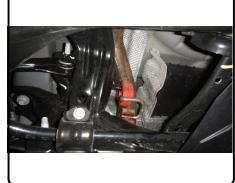
2. Remove the (1) fastener securing the heat shield to the bottom of the driver side frame rail. Trim the portion of the heat shield covering the mounting areas of the driver and passenger side frame rails, see trim diagram. After trimming re-attach the heat shield to the bottom of the driver side.
