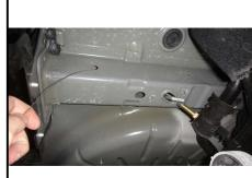
4. Slide the hitch in from the rear passenger side of the vehicle over the exhaust and into position. **Note:** Feed the fishwires through the mounting holes while raising the hitch.
