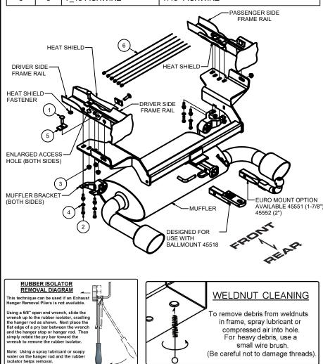
1. Lower exhaust by removing the (4) 8mm bolts from the muffler brackets and the forward rubber isolator. Return the (4) 8mm bolts to the owner.
