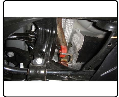
2. Remove the (1) fastener securing the heat shield to the bottom of the driver side frame rail. Trim the portion of the heat shield covering the mounting areas of the driver and passenger side frame rails, see trim diagram. After trimming re-attach the heat shield to the bottom of the driver side.
