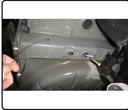
4. Slide the hitch in from the rear passenger side of the vehicle over the exhaust and into position. **Note:** Feed the fishwires through the mounting holes while raising the hitch.
