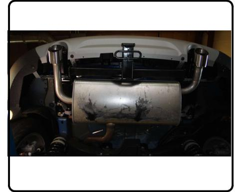
6. Torque all 7/16" hardware to 59 ft-lbs. Torque all M8 hardware to 23 ft-lbs. Re-attach rubber isolator removed in Step 1.
