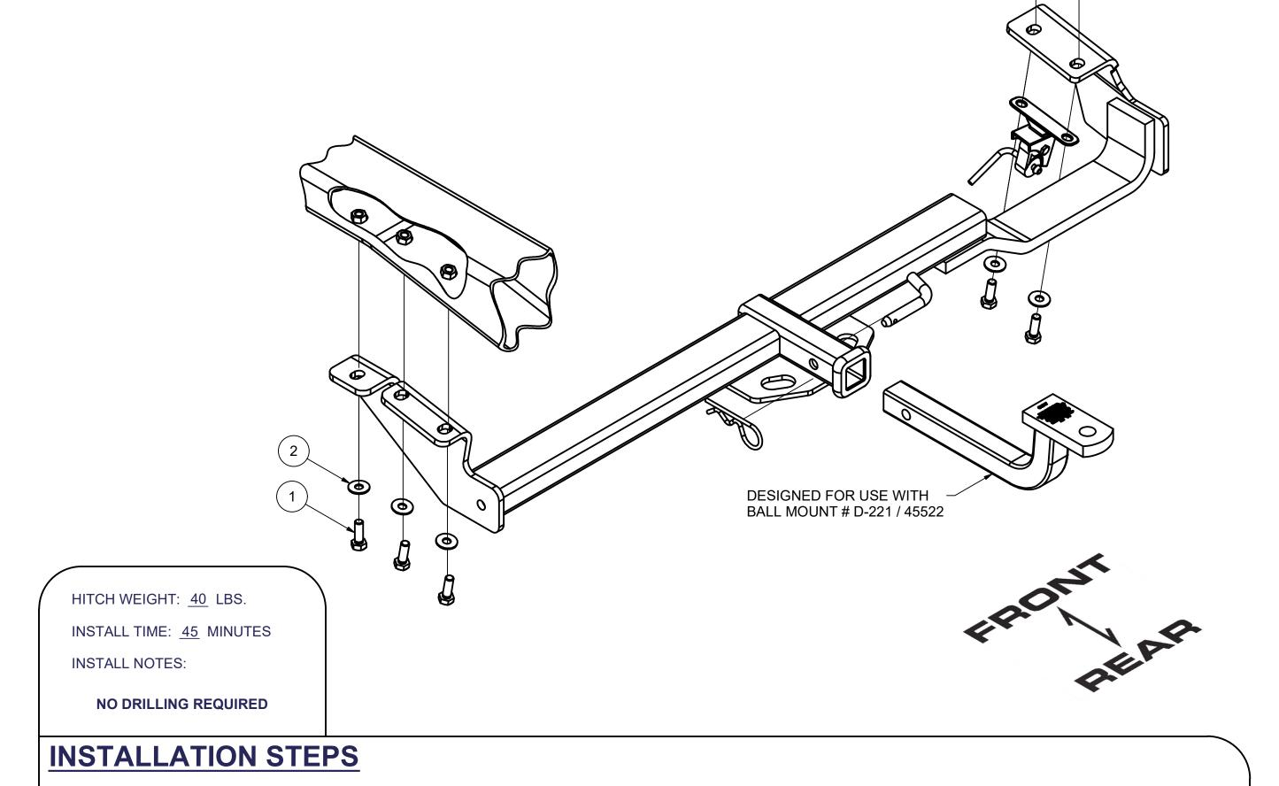
1. If present, remove the tie down brackets and bolts from each side of the vehicle's frame rails. Return these brackets and fasteners to the vehicle's owner.
