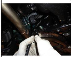
2. Remove (4) heat shield attachments with phillips head screwdiver or 10mm socket (both sides if equipped with dual exhaust). Remove three hole plugs from each side of frame to expose mounting holes. Return all removed items to customer.
