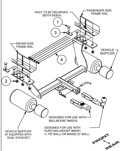
Remove (2) exhaust hangers from the passenger side muffler and (1) exhaust hanger from the center front of vehicle for single exhaust vehicles, dual exhaust will remove (2) exhaust hangers from the driver side muffler as well. Support lowered exhaust with jack stand.
