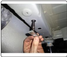
5. Raise hitch into place and secure hitch to frame, using the 1/2" hardware provided. Torque all hardware to 110ft-lb.
