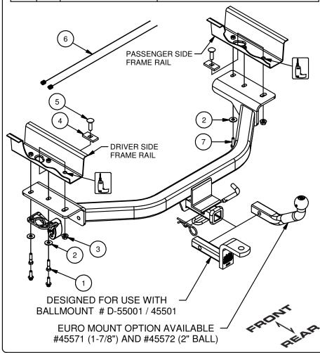
1. Remove (2) bolts and lower the driver side rear exhaust bracket, return bolts to owner.
