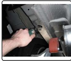
FISHWIRE TECHNIQUE INSERT COILED END OF FISHWIRE TOOL THROUGH HITCH MOUNTING HOLE IN VEHICLE FRAME RAIL AND OUT THE ACCESS HOLE. PASS COILED END OF FISHWIRE THROUGH SPACER AND HREAD BOLT INTO COIL. KINK WIRE O KEEP SPACER SEPERATE FROM OLT AS SHOWN, PULL ISHWIRE, SPACER, AND BOLT THROUGH FRAME AND OUT MOUNTING HOLE. JSE FISHWIRE TO GUIDE HOLE HITCH DURING MOUNTING AND PREVENT LOSS OF BOLT SPACER INSIDE FRAME RAIL. NOTE: SOME VEHICLES MAY FISHWIRE THROUGH END OF FRAME
