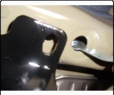
4. Use 1/2-13 hex bolts and 1/2" conical toothed washers and insert hardware through hitch plate and vehicle frame into the handle nut and tighten.
