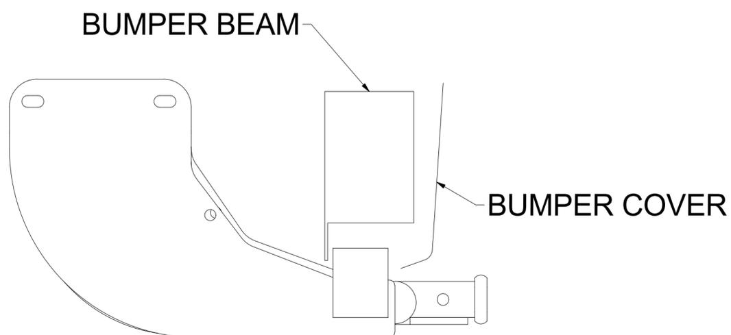
INSTALLED HITCH POSITION
