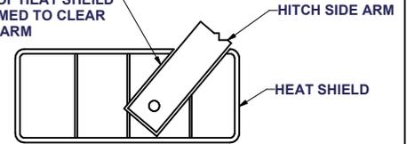
**HEAT SHIELD TRIM DETAIL**
