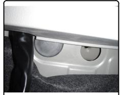
2. Remove tow hook by removing hardware through access holes in trunk pan than remove hardware from underneath vehicle. Put tow hook and hardware in bag and return to vehicle owner.
