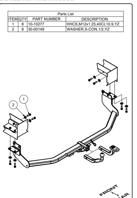
1. Remove two rubber plugs from each side of trunk pan from inside of vehicle. This is done by carefully pulling back the carpet on each side.
