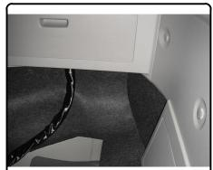
4. Loosely install bolts and washers through access holes in trunk pan. Then torque all M12 hardware to 86 ft-lbs
