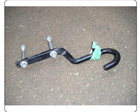
4. Insert 4" hex bolts with washers into the frame rails from the outside. Raise the hitch into position between the frame rails. Push front bolts through mounting plates and loosely install 1/2" flange nuts.
