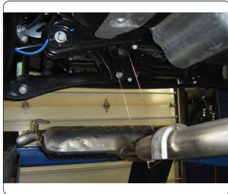
3. Temporarily remove heat shield by removing (4) nuts. (Note: If tow loop is present remove and return to vehicle owner.)
