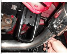
2. Insert 1/2-13 x 4 1/2" carriage bolts and CM-12048-SP spacers through the existing holes in the side of the frame rails. After bolts are inserted push them back so the end is flush with the inside of the frame rails. Temporary lowering of the charcoal canister on the driver side will ease installation.
