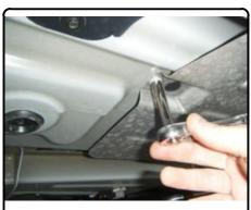
4. Fishwire 1/2-13 x 1 1/2" carriage bolts and CM-SP19 spacers into position through end of frame rails and out mounting holes.
