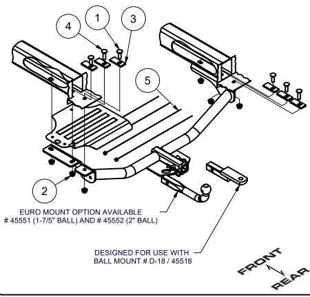
1. Lower exhaust by removing (3) rubber exhaust isolators. Use wire to hold up exhaust to prevent damage to the exhaust tube.
