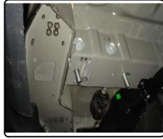
5. Raise hitch into position and secure it with the supplied 1/2" hex flange nuts.
