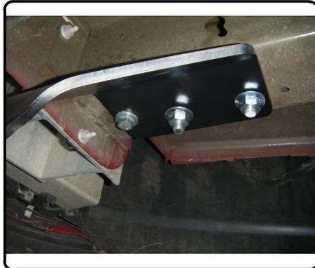
5. Reinstall factory exhaust hanger bracket. Secure using M10-1.5 x 40mm bolts and 3/8" conical toothed washers into existing weldnuts. **Note:** On exhaust side(s) hitch will be sandwiched between the frame rail and exhaust bracket.
