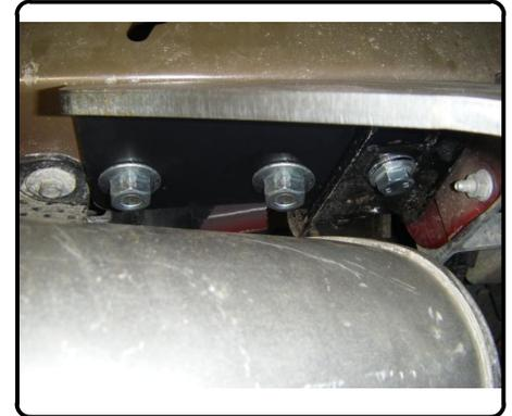
6. Torque all 1/2" hardware to 110 ft-lbs. Torque all M10 hardware to 45 ft-lbs. Raise exhaust back into position.
