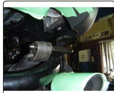
4. Use included hardware to attach hitch and exhaust hangers to vehicle frame. Leave bolts loose. **Note:** Hitch is sandwiched between frame and exhaust hanger.
