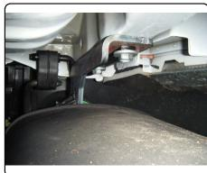
Re-attach (2) center rubber exhaust hangers which were removed in STEP 1.
