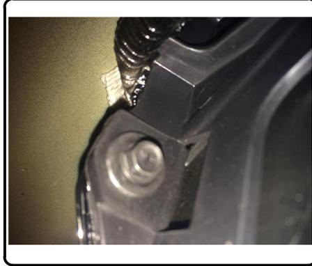
4. Inside the trunk along the plastic liner guard use plastic pry bar to remove (2) caps, (1) on each side, to access and remove (2) T45 bolts, (1) on each side using T45 Torxbit Socket.
