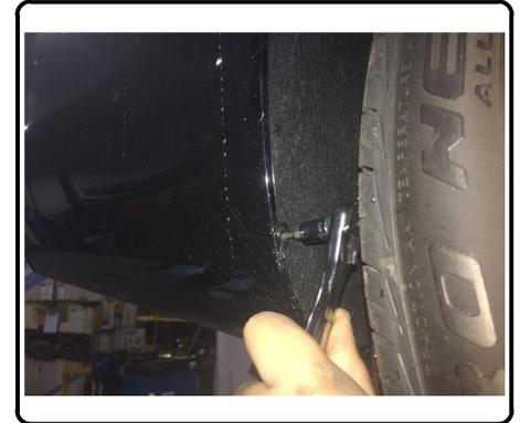
2. Remove (12) M4 screws on the bottom of the bumper fascia using 7mm socket.
