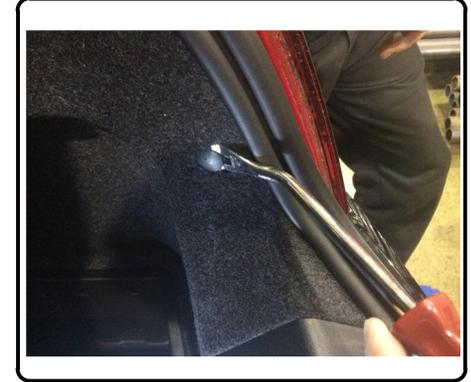
6. To remove taillights, locate and remove (8) M5 nuts using 8mm socket, (4) on each side. Unclip electrical harness and gently remove taillight, set aside for reinstallation in step 12.
