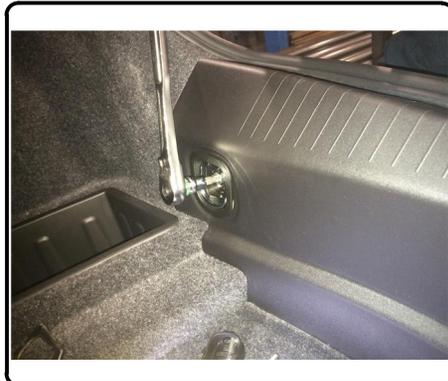
5. Gently remove plastic trunk liner guard and set aside for reinstallation in step 12. Inside the trunk use plastic pry bar to remove (4) plastic clips, (2) on each side, to access taillight removal.
