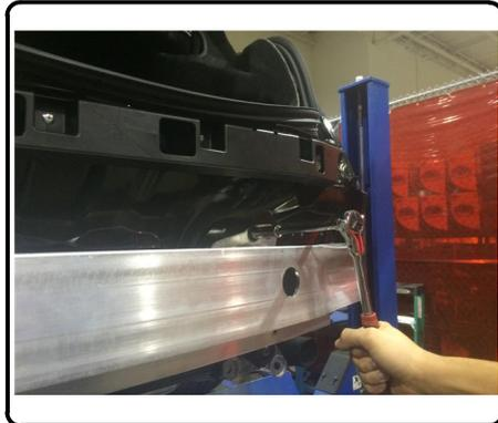
9. Install hitch on rear of vehicle frame using existing studs. Reinstall bumper beam over hitch. Loosely secure with M10 hardware.
