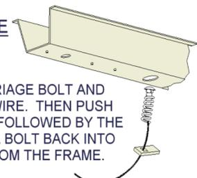
ATTACH FISHWIRE TO CARRIAGE BOLT AND SLIDE SPACER ONTO FISHWIRE. THEN PUSH THE BOLT THRU THE HOLE FOLLOWED BY THE SPACER (AS SHOWN). PULL BOLT BACK INTO POSITION, PROTRUDING FROM THE FRAME.
