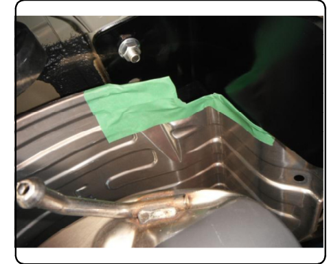
HEAT SHIELD TRIMMING DIAGRAM NOTE: TRIM DIMENSIONS ARE APPROXIMATE, CONFIRM FIT PRIOR TO TRIMMING.
