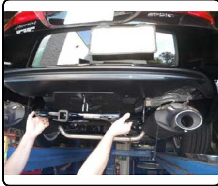
6. Torque all 7/16" hardware to 70 ft-lbs and 3/8" hardware to 45 ft-lbs. (If present) Trim underbody panel then slide hitch bracket through trimmed section. Raise underbody panel into position and reinstall fasteners.
