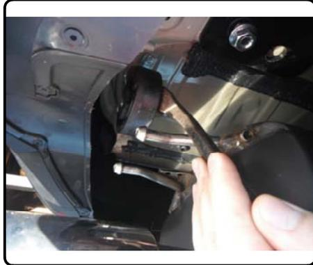
2. Remove heat shield(s) by removing four fasteners per shield. Save fasteners for reinstallation.
