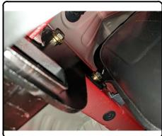
Torque 10mm hardware to 48 ft-lbs. Raise exhaust back into position and secure to vehicle hangers. Reinstall the push pins removed in step 1.
